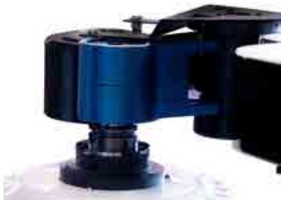
The dedicated cockpit ergonomically integrates the setting and cooling sleeves for an optimized assembly and disassembly process.
