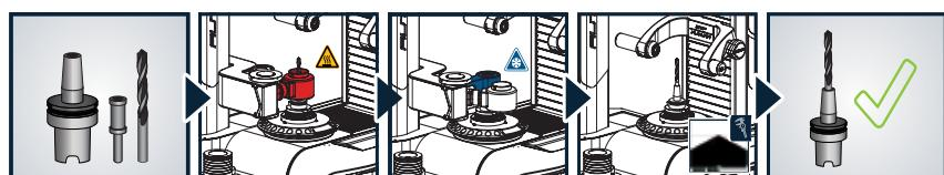
The heating and cooling operations are seamlessly integrated and completely automatic. Operators are guided by a simple step by step process guaranteeing a correct and accurate shrink setup every time.
